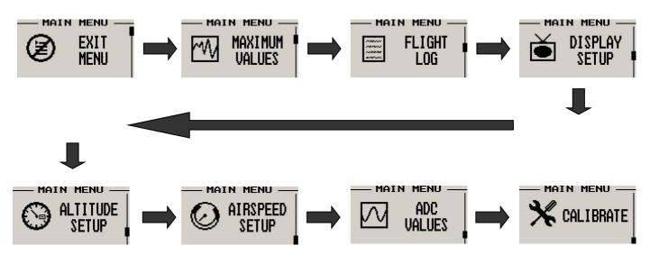
**Note:** (ADC Values and Calibrate Menus are only visible when powering up the unit and pressing the Rotary Control). The text "CALIBRATE" will appear on the intro screen when entering this mode.
